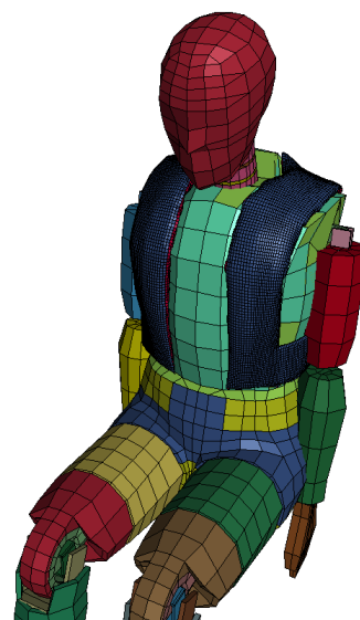
Fig. 6. LSTC's 'Fast HYBRID III 50th Percentile' model with protection provided by air vest protector, inflated using a 50cc carbon dioxide cartridge.
